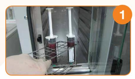
Aseptically withdraw blood using the Orthokine vet irap 60 syringe. Fill syringe, past the soft stop, until plunger locks into place and is flush with the plate and clips. At this point the score mark on the plunger is revealed.
