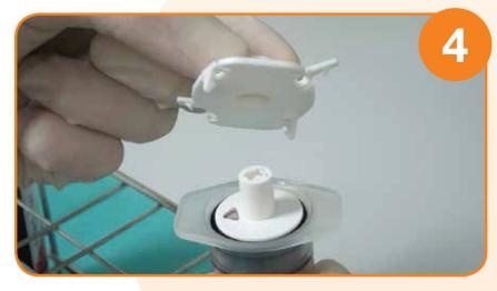
Take off guide plate by rotating it 90°. Place triangular port on the side of the syringe where serum is the deepest by rotating the base of the syringe plunger. Work carefully to not disturb the clot.
